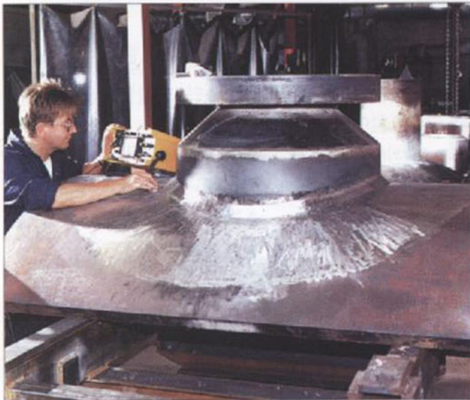
Reactor Vessel Nozzle
