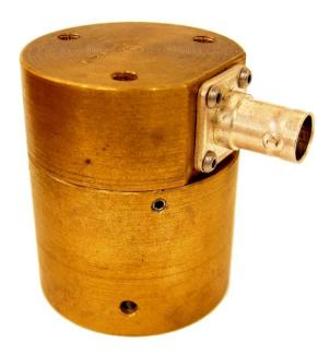
Linearly polarised bulk shear wave probe (LPS3035) for general purpose use, such as with Sonemat's GS2020 EMAT adaptor box system or Sonemat's PR5000 EMAT Pulser-Receiver.
