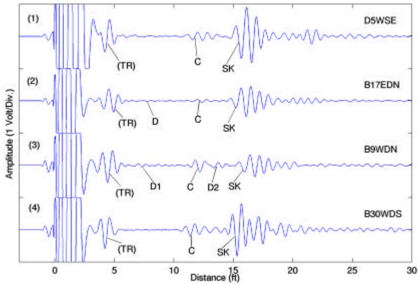
Figure 4. Examples of Data From Socket Side of Suspenders. Top Trace was from a Newly Installed Suspender and the rest were from Old Existing Suspenders.
