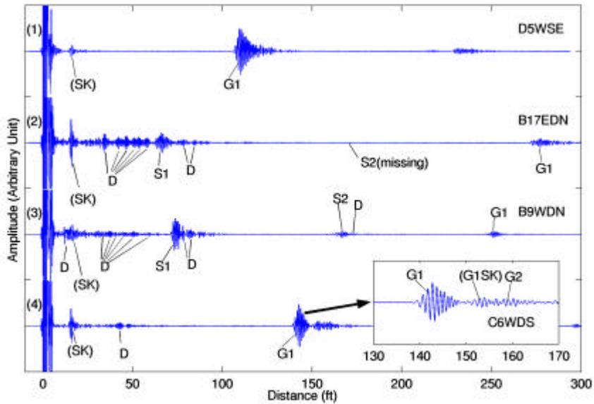
Figure 5. Example of Data from the Main Cable Side of Suspenders. Top trace was from a Newly Installed Suspender and the rest were from Old Existing Suspenders.
