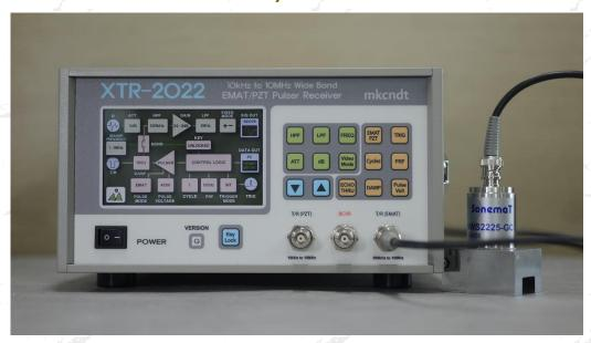
The high-power ultrasonic pulser receiver XTR-2022 developed by MKC is capable of testing in a wide frequency range from 10kHz to 10MHz. For pulse, square pulse method for PZT transducer and square pulse method for EMAT transducer can be used selectively. Therefore, it is a smart device designed to drive the PZT transducer and EMAT transducer in one device, expanding the range of options.
