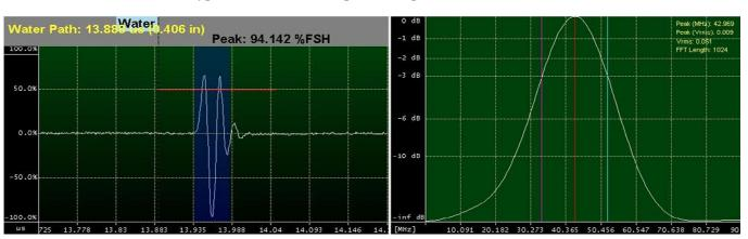
Typical waveform and spectral response is shown below;
