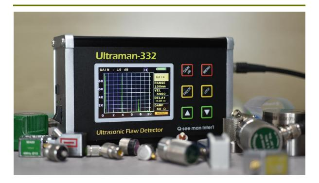
For a long time ultrasonic has been used to find a flaw in hard materials, thickness gaging or to characterize a material in industries. Even now ultrasonic is very useful tool to find crack, porosity, foreign matter, material thickness or characteristics.
