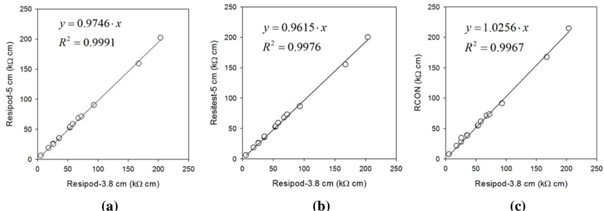
**FIGURE 13 Comparison between bulk resistivity values obtained from different meters with those obtained from Resipod meter with 3.8 cm spacing.**
