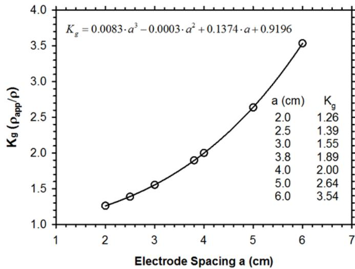
**FIGURE 3 Geometry cell constant for 4×8 in. (10×20 cm) cylinder [8].**
