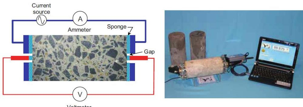
**FIGURE 5 Merlin bulk electrical resistivity meter.**
