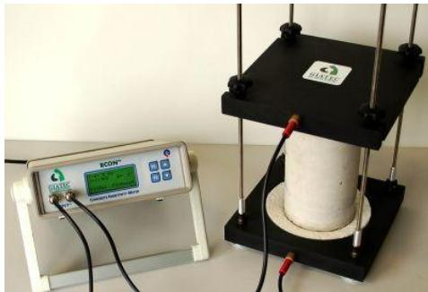
**FIGURE 4 Giatec RCON™ Resistivity Meter for measurement of bulk resistivity of concrete.**
