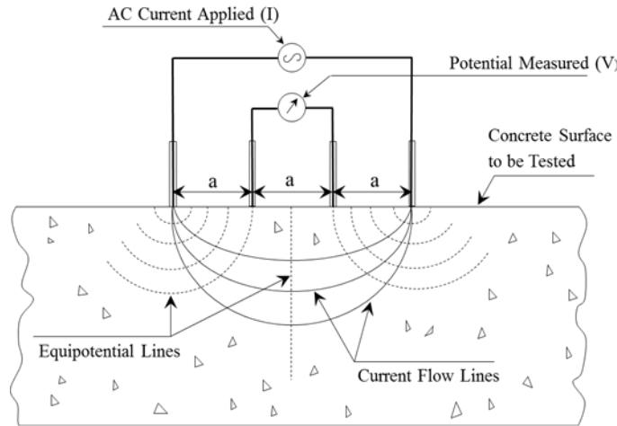
**FIGURE 2 Illustration of the four-electrode (Wenner) method.**
