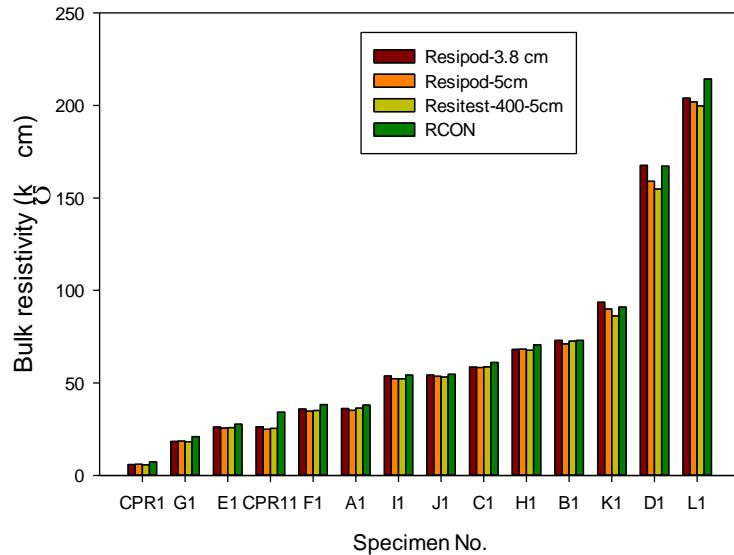
**FIGURE 12 Comparison of bulk resistivity values measured with different resistivity meters.**
