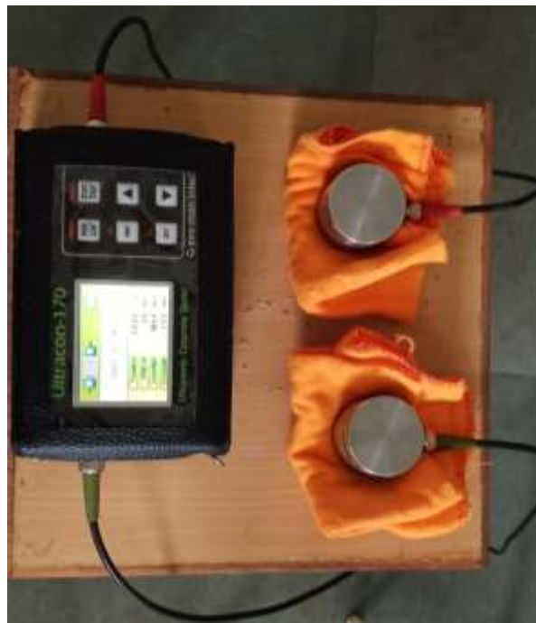
Figure 2: Ultrasonic Pulse Velocity Meter Apparatus Used
