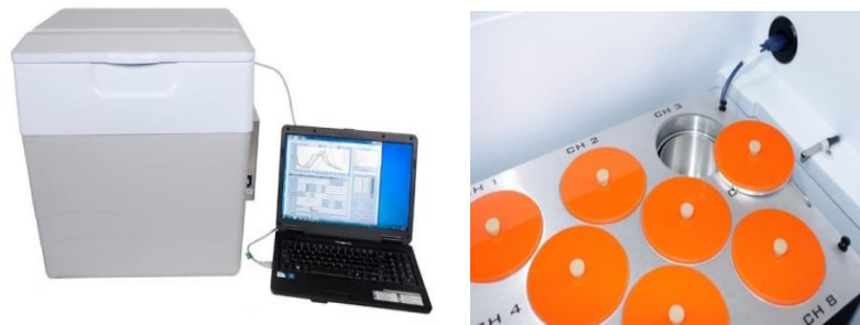
Figure 4.6. Apparatus of Calorimetry Test (Left: I-Cal 8000 with Computer; Right: I-Cal 8000 Interior)
