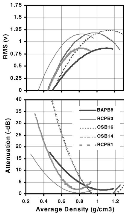
Figure 4. — Least squares quadratic curves of RMS voltage and attenuation versus average density for the five panel types.
