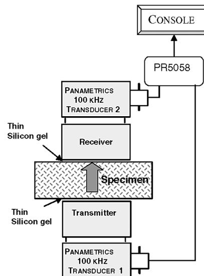
Figure 1. — Experimental setup for the contact ultrasonic system.
