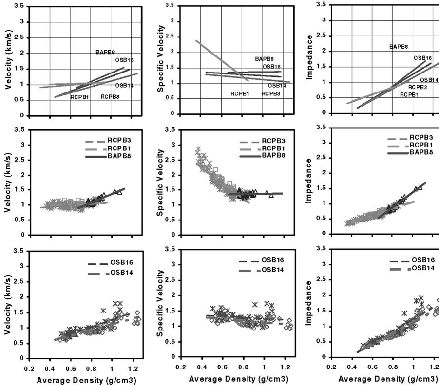
Figure 3. — Least squares straight lines of velocity, SV, and impedance versus AD for five panel types.
