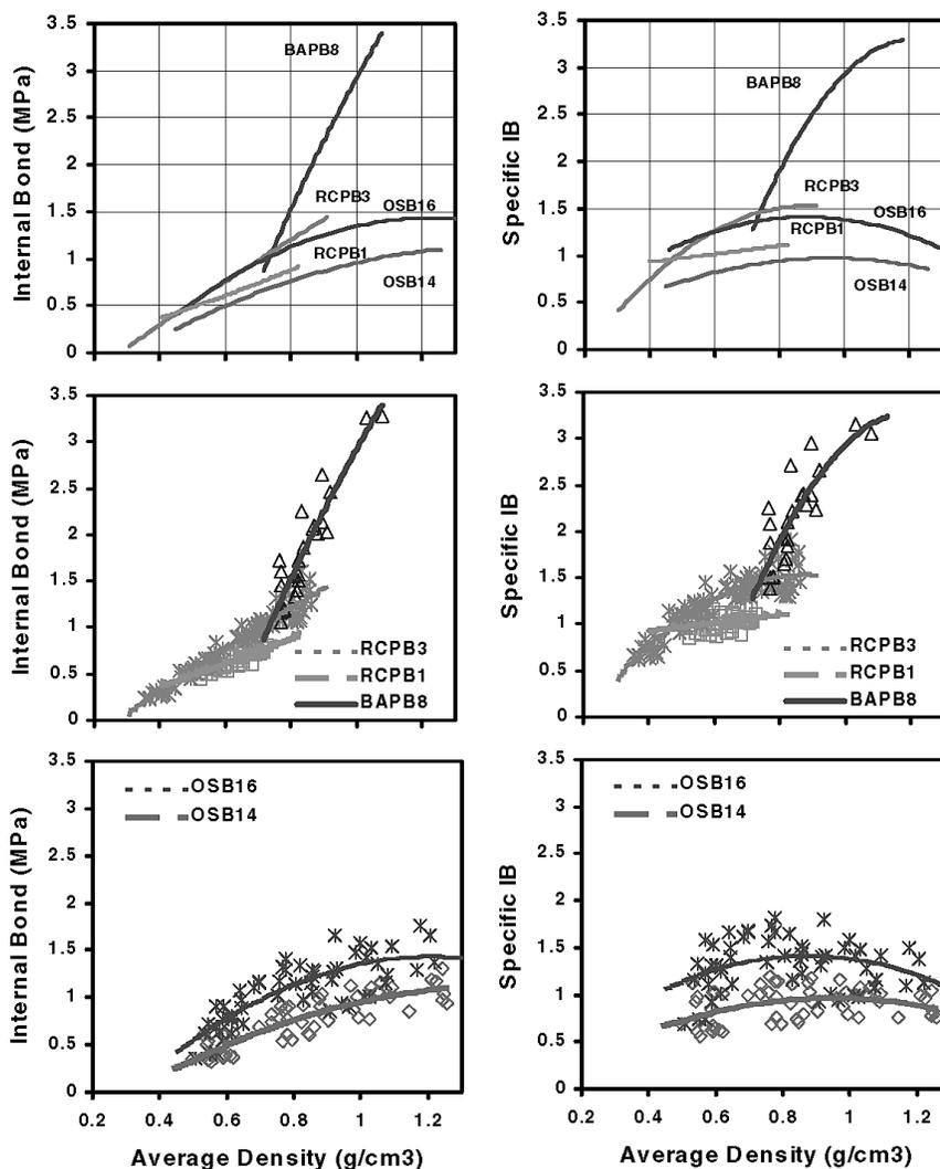
Figure 2. — Least squares quadratic curves of IB and SIB versus AD for the five panel types.
