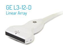
Center Frequency: 6.5 MHz Bandwith: 85% Number of elements: 256 Pitch: 0.20mm Elevation Focus: 22 mm Elevation aperture: 5.0 mm
