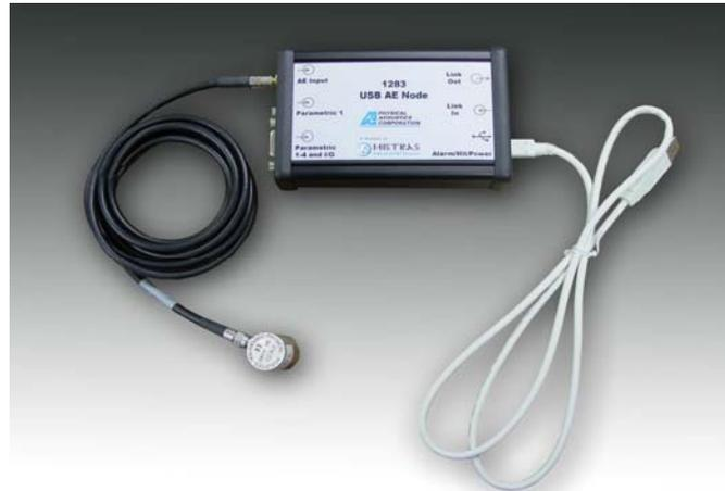
**Figure 2.** USB-AE Node and Accessories
